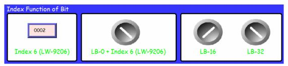
If Index 6 (LW-9206) is set to 2, then switch [LB-0 + Index6] reads LB-32 which is in OFF state.
