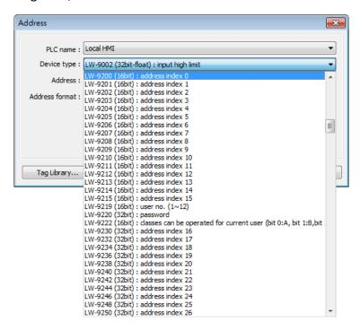
The corresponding address of 16-bit Index Register 0 to 15: LW-9200 (16bit) to LW-9215 (16bit) The maximum offset range is 65536 words.
