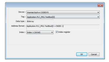
Note that, unlike its non-tag counterpart, the 16-bit offset is not necessary for Bit array tags.
