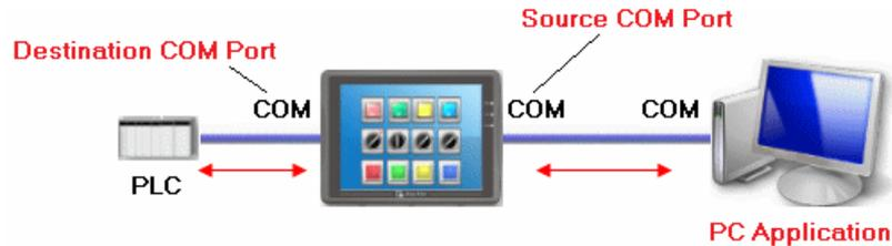
**[Source COM Port]** The port connects HMI with PC.
