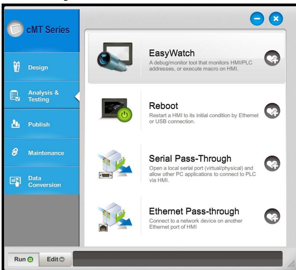
2. Click [Ethernet Pass-through] and then fill in the communication parameters.
