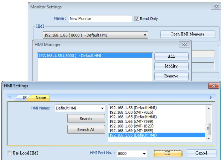
Or, select [Use Local HMI] checkbox to use the project on PC as a monitoring device.
