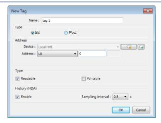
Add a new tag for the client to monitor or control. The name must be entered, and the address can be Readable or Writeable.
